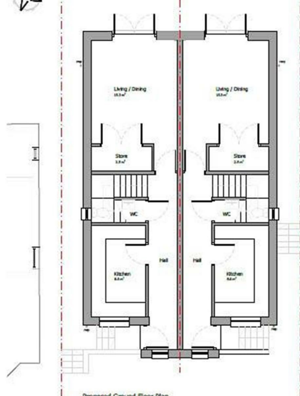
Proposed Ground Floor Plan Scale 1:50 Each Plot GF GIA - 42.3sqm Each Plot Total GIA - 91.3sqm
